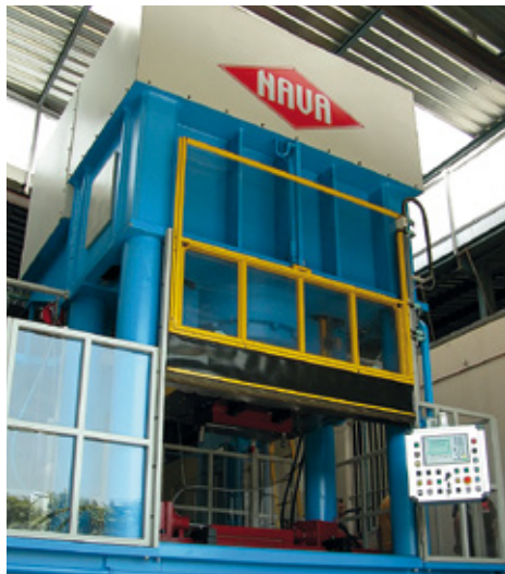
Hydroforming press for collections of large tubes, typically exhaust pipes for the motorbike sector, designed and produced by F.lli Nava.
